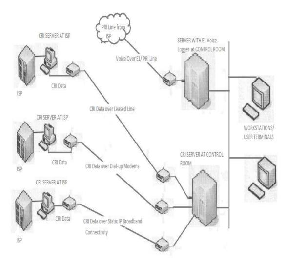
Our system has facility to integrate Call Related Information/Data available at ISPs at central location with the Digital Voice Logger as shown in configuration diagram above. It is an optional feature and is not available with the standard system.
