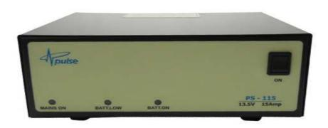
PS-115 is a light, compact, reliable and efficient SMPS Power Supply cum Battery Charger Unit. Operating on Single Phase Mains Input, it delivers 15Amp Current at 13.5Volt DC. It is meant for use in VHF/UHF Radio Transceivers systems. Apart from facility of automatic switching to battery power in case of mains failure, it also has protection against short circuit, overload and output over voltage.
