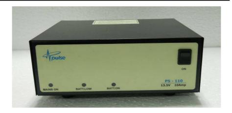
PS-110 is a light, compact, reliable and efficient SMPS Power Supply cum Battery Charger Unit. Operating on Single Phase Mains Input, it delivers 10Amp Current at 13.5Volt DC. It is meant for use in VHF/UHF Radio Transceivers systems. Apart from facility of automatic switching to battery power in case of mains failure, it also has protection against short circuit, overload and output over voltage.
